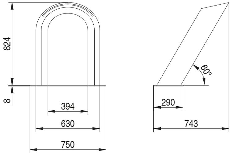
CASCADA MINI BOW · WATER CURTAIN MINI BOW · CASCADE MINI BOW
